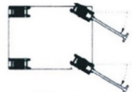
METHOD 2 2 straight cargo trolley + 2 steering cargo trolley
